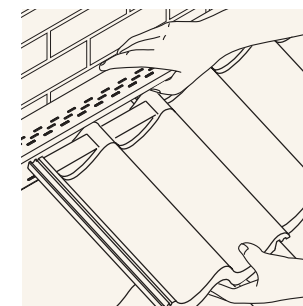
Insertion of profiled tiles into batten section
